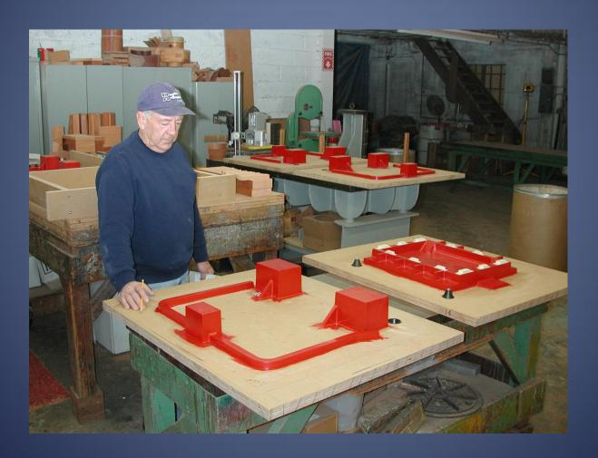
Chemical sand binders can degrade plastic tooling.
